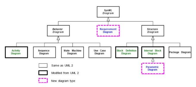
Fig.1 The nine diagrams according to the four pillars of modeling in the SysML language
