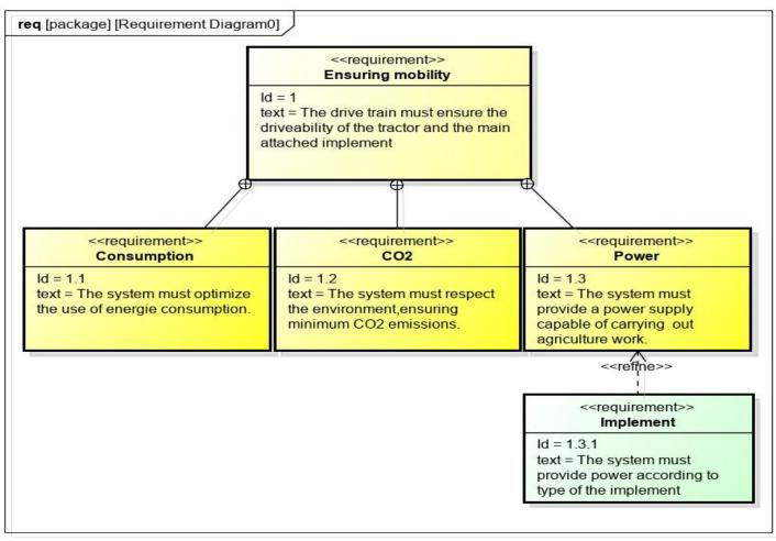
Fig. 2 Requirement diagram of the drive train of the low-cost tractor.
