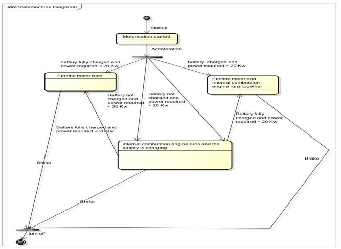
Fig. 5 StateMachin Diagram of the drive train of the low-cost tractor.
